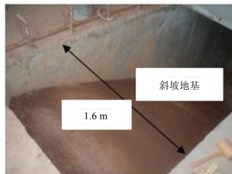
图2 试验模型槽 Fig.2 Test cavity in Lab
